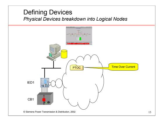
To return to our substation architecture, IED1 is a multi-function IED and supports the following features:
