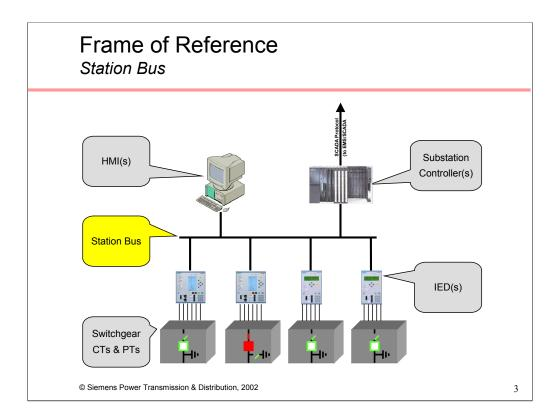
The goal for numerous years has been to define a communications infrastructure that will allow seamless integration of the IEDs into higher level devices - an infrastructure that is vendor independent and will allow devices from multiple vendors to be integrated together. The definition of a suitable Station Bus as depicted above has been the focus of standardization efforts on both sides of the Atlantic.
