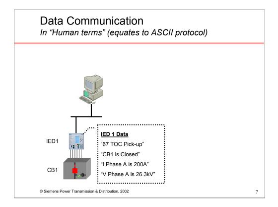
To explain some communication concepts, we'll use a simplified version of our substation architecture – an HMI connected to one IED.
