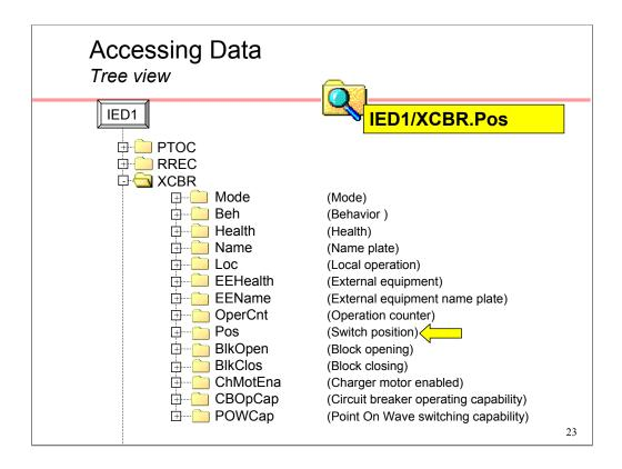
The XCBR LN consists of 14 "folders". The **Pos** "folder" contains information about switch position, so this would be drilled-down into.
