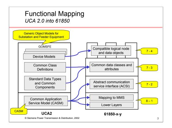
This rather daunting looking diagram extracted from the IEC 61850 specification depicts the mapping of the Application layer of UCA 2.0 into 61850.
