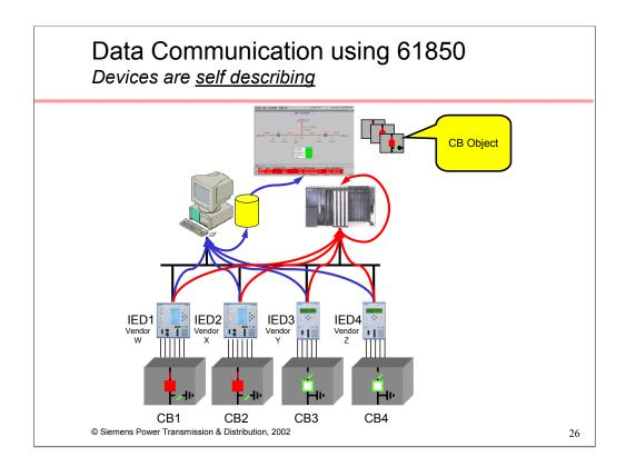
The remainder of the system is configured in the same fashion. Data from the other IEDs are available to the HMI and Substation Controller for incorporation into one-lines, historical archives, control sequences, logic programs, automation applications, etc.
