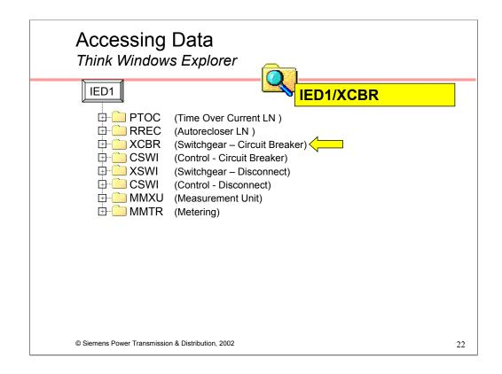
Accessing data in a 61850 network is analogous to accessing data across a conventional IT network using Windows Explorer, i.e. browse the network until the data source is located, then drill-down into the data source until the data is located.
