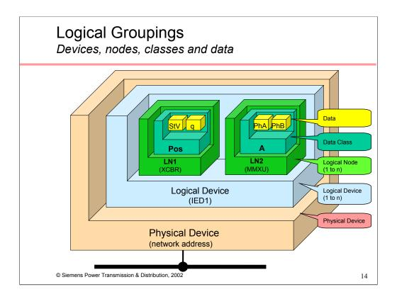
The container is the Physical Device, it contains one or more Logical Devices, each of which contains one or more Logical Nodes, each of which contains a pre-defined set of Data Classes, each of which contains data.
