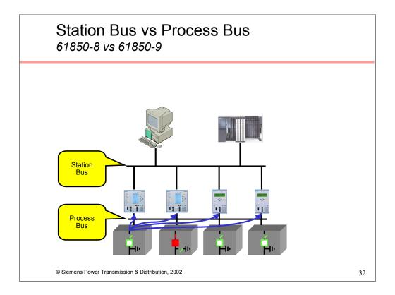
The Process Bus replaces hard wired connections with communication lines. "Smart" CTs, PTs and switchgear continuously transmit data over the process bus and any upstream devices that wish to use the data for protection, measurements, metering or monitoring do so by monitoring the communications.
