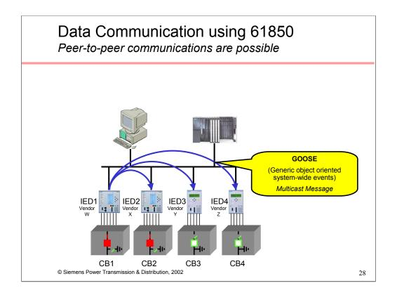
GOOSE is an acronym for Generic Object Orientated System-wide Events. It aims to replace the conventional hardwired logic necessary for intra-relay coordination with station-bus communications. Upon detecting an event, the IED(s) use a multi-cast transmission to notify those devices that have registered to receive the data. The performance requirements are stringent – no more than 4ms is allowed to elapse from the time an event occurs to the time of message transmission.
