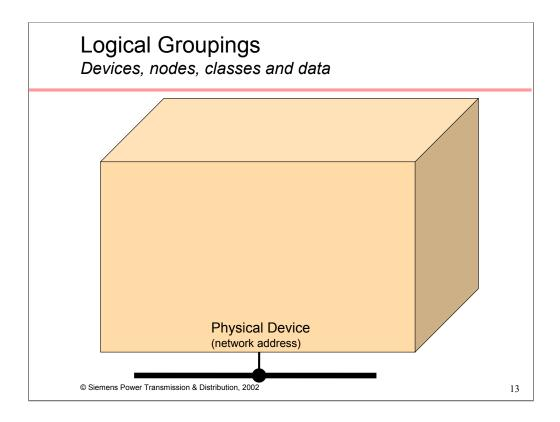
To illustrate how these device, logical nodes, classes and data concepts map to the real world, imagine an IED as a container.
