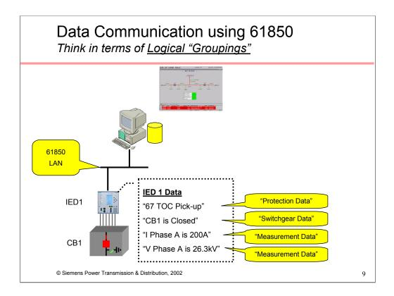
Instead of dividing data into I/O types like Digital Input data, Analog Input data, etc, as is the case with DNP 3.0, IEC 61850 divides data into <u>logical groupings</u>. So in our example above we have:
