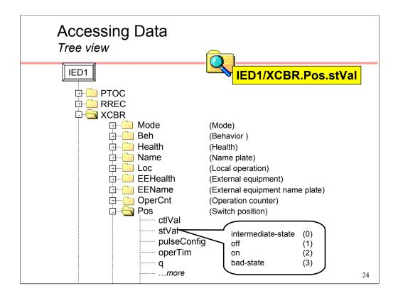
The **Pos** "folder" is of type Controllable Double Point (CDP) data class. The CDP data class consists of 14 data fields (some are mandatory and must always be present, others are optional). The **StVal** field contains the value of the CB.
