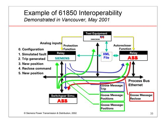
The above diagram illustrates how 61850 is used in a "real world" example in a recent interoperability demonstration.
