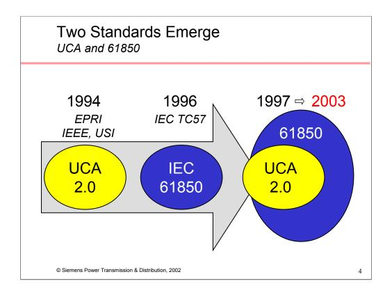
EPRI and the IEEE spear-headed an effort to define an Utility Communications Architecture (UCA) beginning in the early 1990s. The initial focus was inter Control Center communications and Substation to Control Center communications. This culminated in the ICCP specification which was later adopted by the IEC as 61850 TASE.2.
